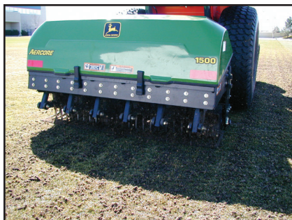
Example of a sports field being aerified. Photo: Ross Kurcab, CSFM
